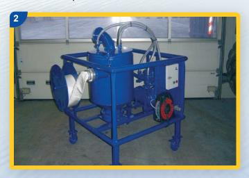
This specially constructed adapter is required for the changeover from silo trucks to a silo rail car (1) in closed system. The adapter filters the exhaust air by means of a specific filtering unit.
