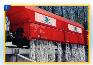
These slag rail cars are employed for the transport of slag resulting from refuse incineration plants. The loading is achieved by means of a tipping process or gravity.
