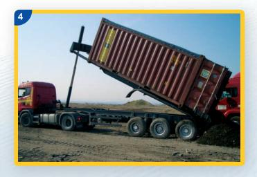
These open top containers are available in 20 or 30 foot designs and are employed to deal with contaminated soil when the evacuation can be undertaken by dumping the contents of the container into the landfill.
